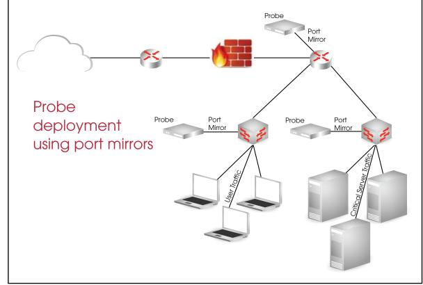
A network device can support a restricted number of port mirrors. This limitation is increasingly important as more security and analysis devices try to access the same data.
