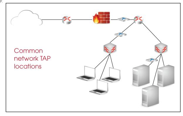
throughout the network. The passive nature of TAPs, ensure that network communication is maintained. Combining TAP outputs with the use of an aggregation device means greater visibility for the network probe.
