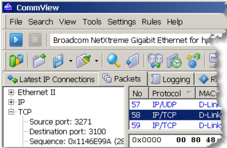
the industry. This application captures every packet on the Ethernet wire (or dial-up connection) to display important information such as a list of packets and network connections, vital statistics, protocol distribution charts, and so on. With this information, CommView can help you view and examine packets, pinpoint network problems, and troubleshoot software and hardware.
