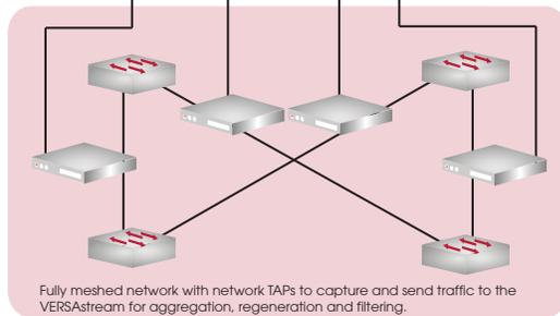
Fully meshed network with network TAPs to capture and send traffic to the VERSAstream for aggregation, regeneration and filtering.
