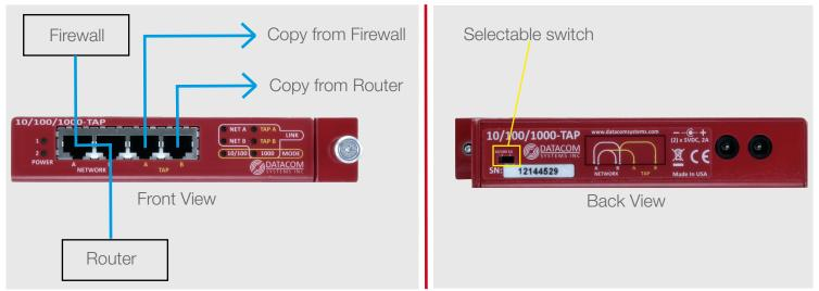
A convenient switch on the back of the tap can be used to select the tapping mechanism, either a 1G network link or a 10/100Mbps link. All devices connected to the tap should be capable of the same maximum speed.
