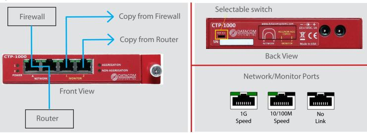
A convenient switch on the back of the tap can be used to toggle aggregation on or off. When set to "NON", Monitor port A will only transmit a copy of received traffic on Network port A, and Monitor port B will only transmit a copy of received traffic on Network port B.
