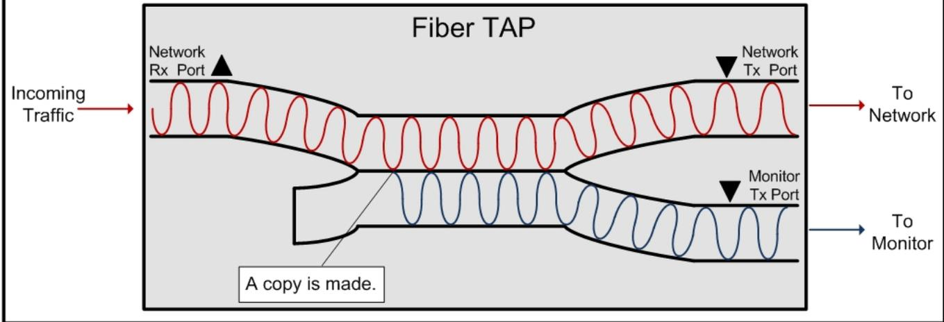
**Reverse Wiring:** If the fibers are connected backwards, light will not be received on the monitoring port. This is because the internal coupler that splits the light is unidirectional.
