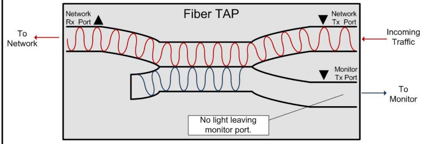
**To Avoid Reverse Wiring:** Reverse wiring can be difficult to catch initially, since an incorrectly cabled Fiber Tap will still send light between the network ports and connectivity will be seen on both network endpoints. Be sure to check for light on the monitor ports as well as the network ports when installing the Fiber Tap.
