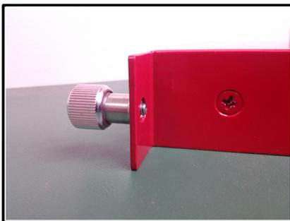
Use the thumbscrew on the other end of the Datacom device to screw it into the rack mount.
