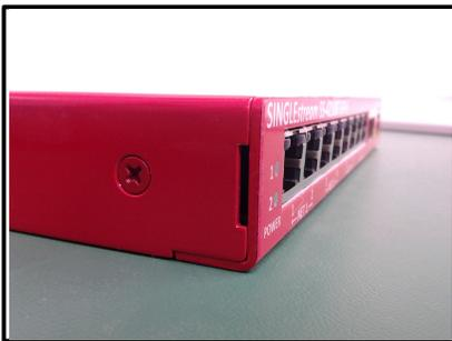
Notice that the Datacom Systems device has a notch on the left side. This notch is used to hold the device until it is screwed in.
