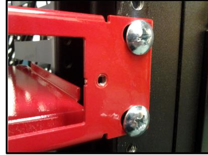
Once the holes on the rack mount and the rack are lined up, use four screws to secure it to the rack.
