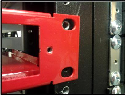
Determine the location on the rack that the taps are to be installed. Line up the mounting holes on each side of the rack mount with the holes on the rack.
