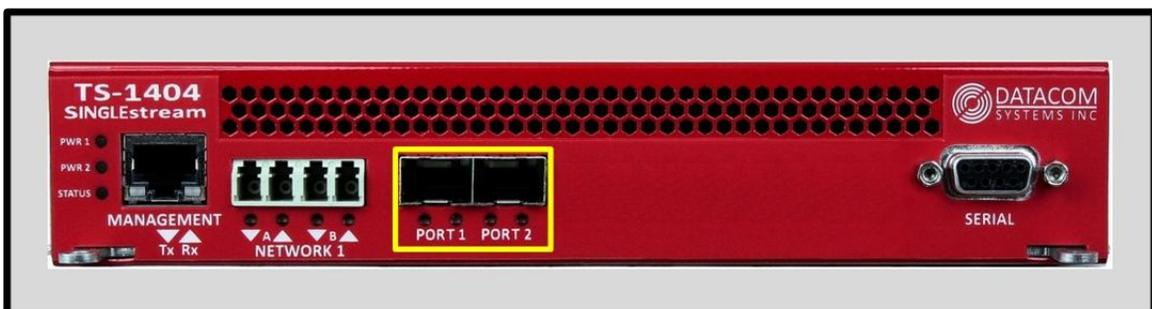
**Serial Port:** The serial port can be used to connect to the SINGLEstream™ Aggregation Tap using a DB9 M/F straight through cable. Using a terminal emulator such as Tera Term or Putty, the serial port may be accessed for login and configuration using the CLI interface.
