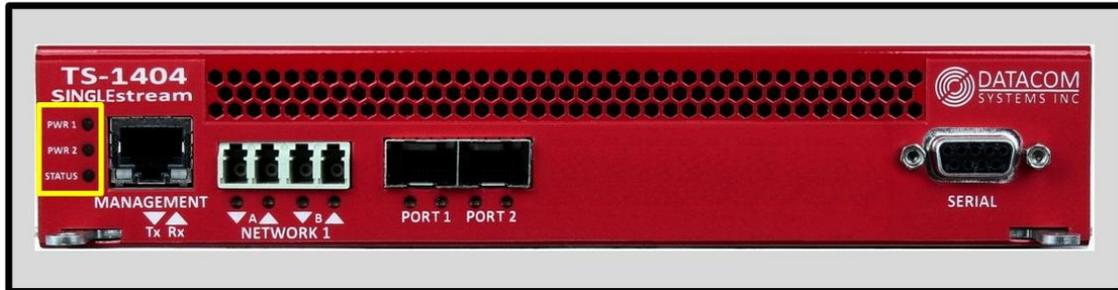
The LEDs located next to each power label will illuminate **green** when an active power supply is connected.
